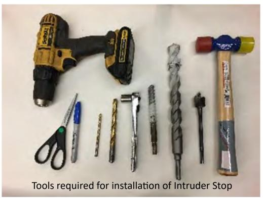
Scissors, marker, tape, ¼" drill bit 3/8" drill bit, drill motor, hammer drill motor for concrete, 9/16" wrench or socket, hammer (recommend plastic), ½" and 1" carbide drill bit for concrete (a 1" coring bit works best) or 1" boring bit for wood.
